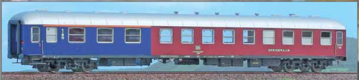
Carrozza DB ARmh 216 "Speiseraum" con scompartimenti di prima classe e area ristoro in livrea blu/rosso. DB Type ARmh 216 "Speiseraum" car, with 1 st class compartments and refreshment area. Blue and red livery. DB Schellzugwagen Typ ARmh 216 mit 1. Klasse Abteil und Speiseraum. Lackierung in blau und rot.
