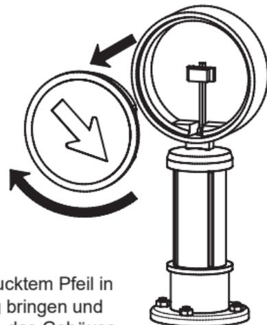
*Rotate the front panel with the arrow to the desired direction and press it slightly to fasten it.*
