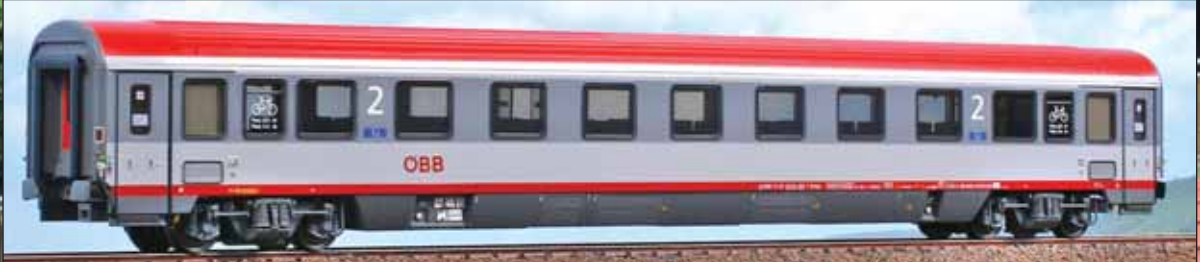
Carrozza Bmpz di 2ª classe a salone, in livrea "Upgrade", con carrelli SGP. 2 nd class Bmpz saloon car, in "Upgrade" livery, with SGP bogies. Bmpz-Salonwagen 2. Klasse, in „Upgrade“-Lackierung, mit SGP Drehgestellen.
