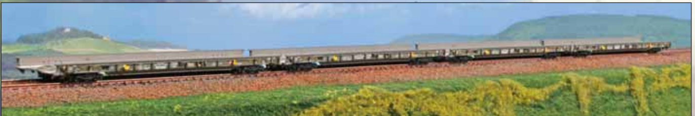
Set Rollende Landstraße HUPAC composto da quattro carri Tipo Saadkms per trasporto di camion. Rollende Landstraße HUPAC set composed by four Type Saadkms wagons for truck transport. Rollende Landstraße Set HUPAC bestehend aus vier Typ Saadkms-Wagen für den LKW-Transport.
