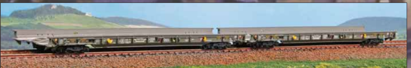
Set Rollende Landstraße HUPAC composto da due carri Tipo Saadkms per trasporto di camion. Rollende Landstraße HUPAC set composed by two Type Saadkms wagons for truck transport. Rollende Landstraße Set HUPAC bestehend aus zwei Typ Saadkms-Wagen für den LKW-Transport.
