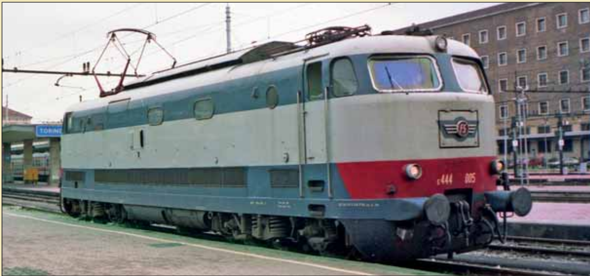
Locomotiva elettrica E.444.005 ex "elettronica" ricostruita come unità di serie. Electric locomotive E.444.005 former "electronics" rebuilt as a production unit. Elektrolokomotive E.444.005 Ehemalige "Elektronik" als Serieneinheit rekonstruiert.
