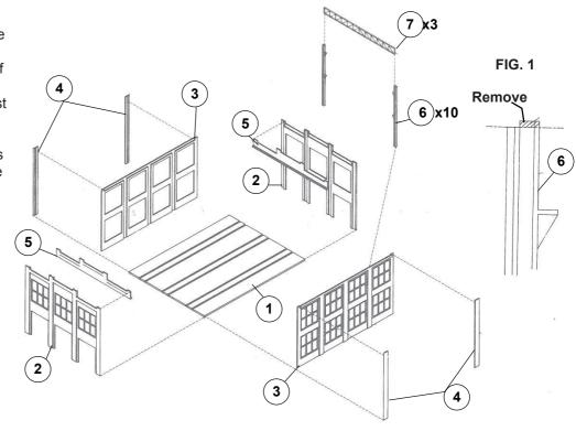
2. First, glue end pilasters (4) to the side walls (3). Next, glue five support columns (6) to the inside of each end wall. NOTE: The support columns that go in the corners must have their tops removed (see fig.
