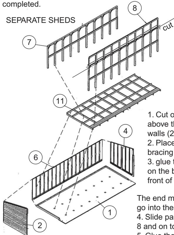
1. Cut off the top section of part #8, just above the "V" bracing. After gluing the walls (2, 4, 6) to the base (1).
