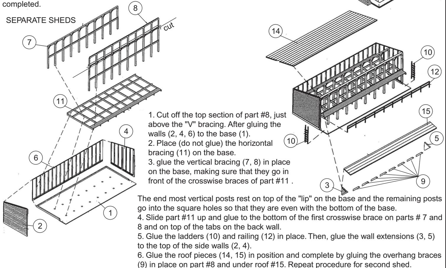
1. Cut off the top section of part #8, just above the "V" bracing. After gluing the walls (2, 4, 6) to the base (1).
