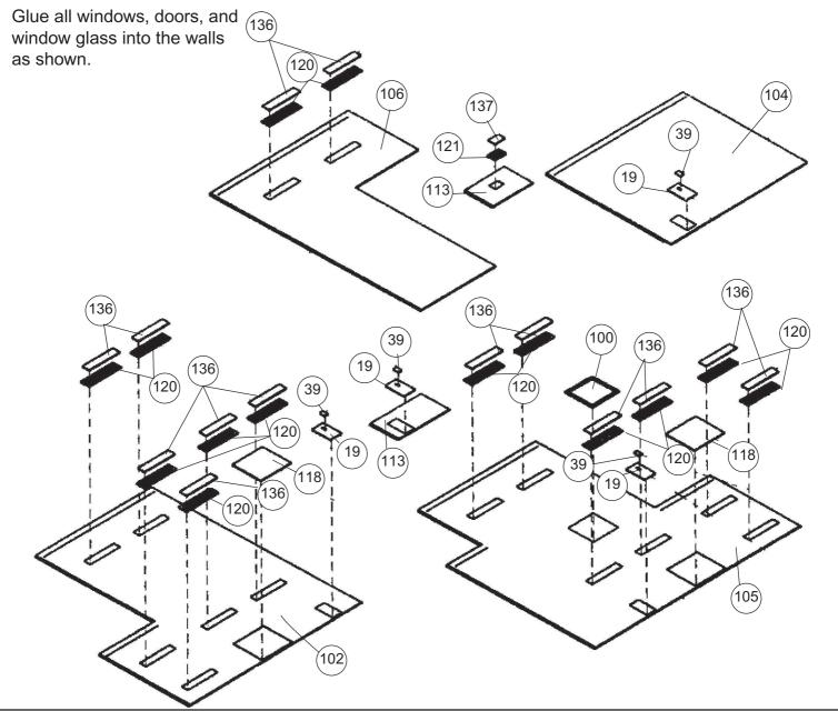
Glue Walls (102, 103, 105, 106, 107, 108) to the base (101). Glue Wall (104) to top of walls (102, 105). Drill holes on bottom of Roof (109) for the number of stacks and vents desired. Glue roofs (109, 110, 111) in place.
