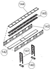
Glue pipes (145) to floor of bridge (142), one set of pipes on top of the others. Glue the sides (143) and top (144) on. Glue the supports (141) to the pads (140) and finish the bridge by gluing the supports to the bottom of the floor.
