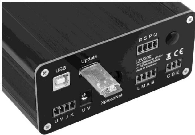
Now switch on the power again (plug in the screw terminal U,V,J,K again). The lower LED on the front of the LZV200 flashes.
