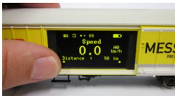
The display shows the actual measurements being taken, their value, and activated functions; i.e. "test run active."
