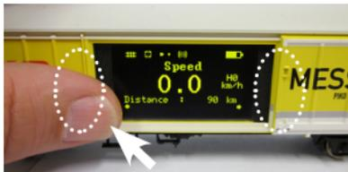
There are touch-sensitive black vertical panels located to the left and the right of the display. Place your fingertip on one of the panels marked in the photo for a half-second. The display will switch back and forth between different screens or different functions (see section 2.3). The small yellow arrows at the lower edge of the display indicate whether another screen can be accessed.
