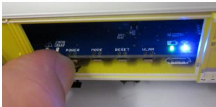
To turn off the PIKO SmartMeasure Car, press the POWER key for seven seconds. If the car is not sitting on live track or is not moved for 3 minutes, it switches off automatically.
